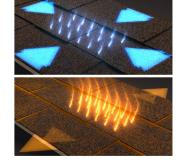
Fluctuations in weather and temperature cause asphalt shingles to expand and contract significantly, even within a given hour. It's the natural oils in the asphalt that allow these expansions and contractions to happen while your roof protects your building as it should. As the shingles age, though, this oil evaporates, causing them to dry out and lose their flexibility, as well as their top protective layer of granules.
